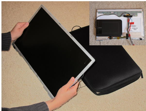
Figure 2.1: Device setting: (1) Participant, (2) 17 inch BackPad (we.e. semi-detached laptop screen), (3) Monitor cable, (4) Bamboo touch-pad
